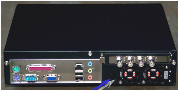
DC power, camera and network inputs (Photo may vary, cameras not included)
