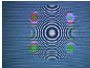
Color fringes in inferior composite video (NTSC)
